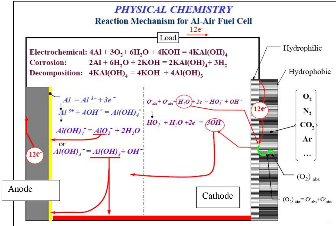
Fig. 1. Reaction mechanisms for aluminum-air fuel cell
